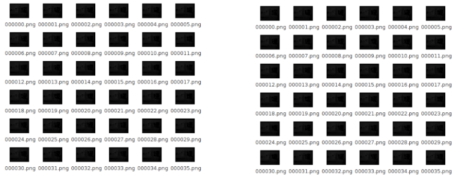
Figure 6.5: The datasets folders depth (left) and 3_depth (right) that hold the two views of our simulated 16-bit depth renderings of our ground truth. File managers typically expect 8-bit png images so the 16-bit depths may appear black until processed by a proper PNG reader.
