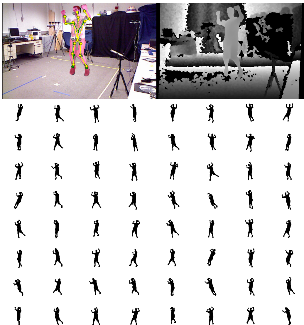
Figure 3.1: Top Left: Highlighted solution over an observed frame. With green color we have highlighted the correct location of each of the body joints which is our ground truth. With gray color we have highlighted the joint positions as estimated by the chosen Neural Network Discriminative human detector. Although they are not totally inaccurate they are still relatively far away from the true solutions. With Yellow we can see the joint colors that have been refined using a generative method that are much closer to the correct solution and thus mostly occlude the green markers. Top Right: The observed Depth Map contains both background and foreground. Thus a generative component would find correspondences with other objects in the scene as well as our target, discriminative methods on the other hand given enough training can completely reject background and are much less prone to false positive results. Bottom : A batch rendering of 64 random configurations of a human body that adhere to our movement limits and are close to the previous known configuration. The depth color has been inverted to make the figures more visible. Our configurable 3D body model will be used to form such hypothesis that will be iteratively scored, assessed and refined until we converge to the good solution shown top left.
