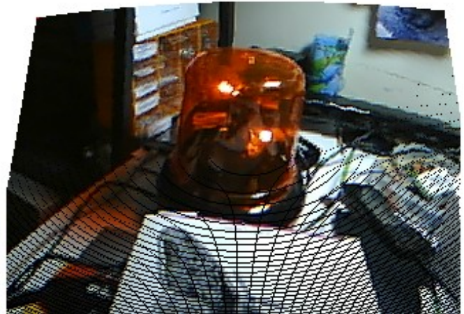
Illustration 9: Raw images received from the cameras and their calibrated equivalent ( the distortion parameters are exaggerated to better show the way calibration alters the input images )
