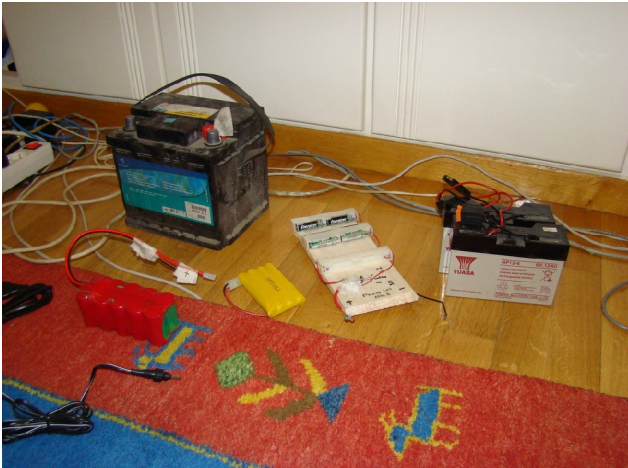
Illustration 57: Battery types tested, none fitted the cost/weight-energy requirements of GuarddoG but NiMH was the chosen chemistry
