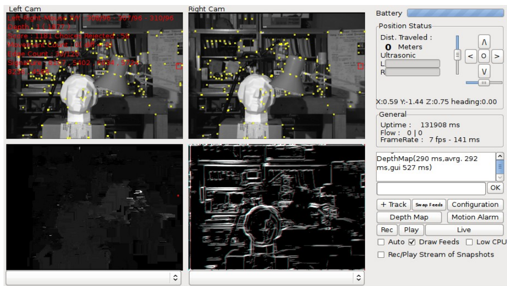
Illustration 26: Disparity Mapping on the GUI of Guarddog
